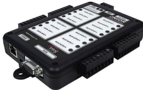
JNIOR runs Task Manager and can also interface with applications on other computers via TCP/IP packets, Modbus/TCP, OPC server, Windows API (DLL) or Web services at the
