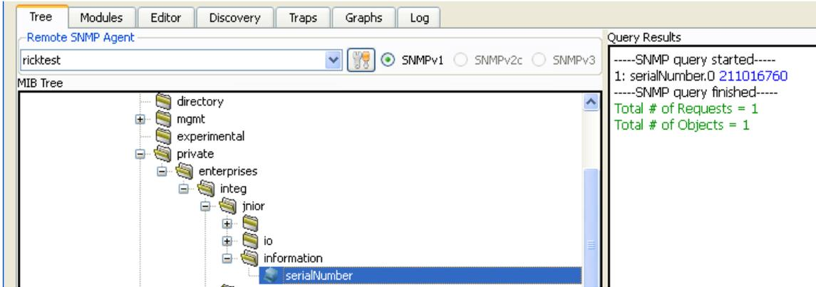
The user can query the status of each input and output either as a 'mask' (one number that represents the status of all inputs or outputs - decimal number based on binary representation of 1's and 0's for each input or output) or the status of each individual input or output.
